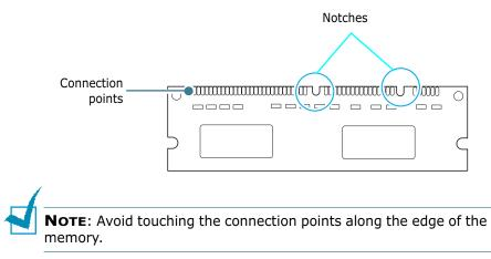
7 Holding the memory DIMM by the edges, align the notches on the memory DIMM with the notches at the top of the memory DIMM slot.
